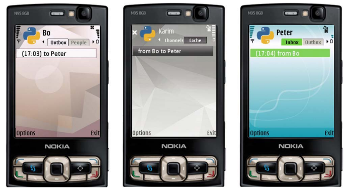
Fig. 1. Snapshots of the user interfaces in a demo scenario (Bo initiates a message addressed to Peter, who is out of direct contact of Bo. Karim, who meets Peter more often, carries the message from Bo, and delivers it to Peter when he encounters Peter again.)
